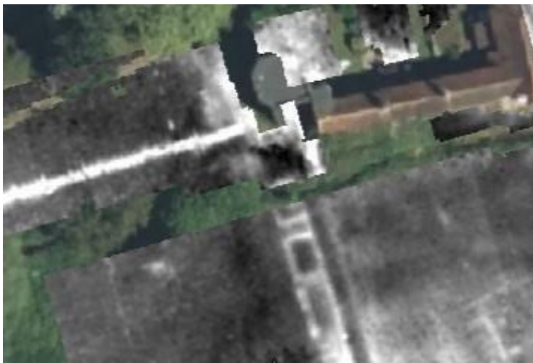
Figure 26: Resistivity survey 2023. The NW Tower is in the top centre of the image. Areas of high resistivity (white) can be seen surrounding the Tower. The linear line running to the left (west) is a known buried conduit, and the buried foundations of the western range can be seen running south of the Tower. (Image courtesy of Anne Sassin and DVLP)
